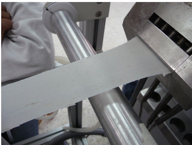
Figure 4.1 Flexible film based on cassava starch obtained by extrusion
