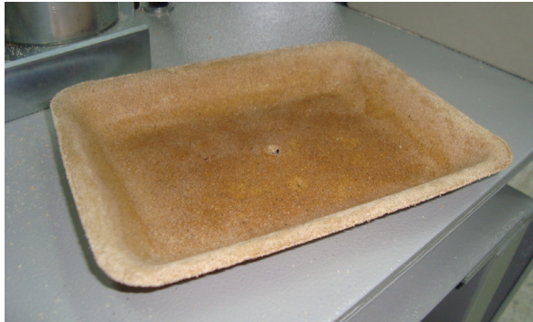
Figure 4.2 Semi-rigid tray based on cassava flour created through thermocompression
